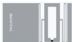
MidasFlagTag (Monza R6-P) (W)31.41mm×(L)18.0mm
